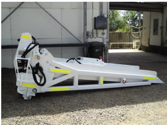
Underground Cassette Racker, Repaired including Statutory inspections and reporting for Rio Tinto.
