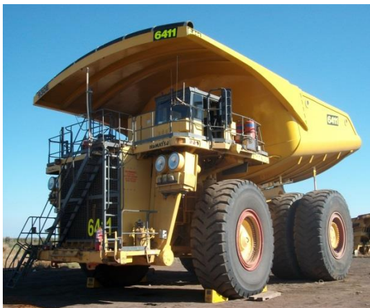
Komatsu 930E Tray rebuild carried out onsite.
