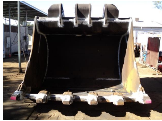
250 ton Excavator Bucket rebuild including new Adaptors and GET, Heel Plates, Crack Repairs and Line Boring.
