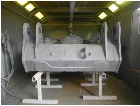
Kress Hauler Swing Frame sandblasted ready for Paint. Refurbishment and strengthening kit added As per OEM Specifications.
