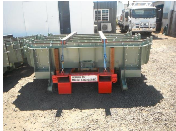
New Reclaimer Shovels fabricated for BMA
