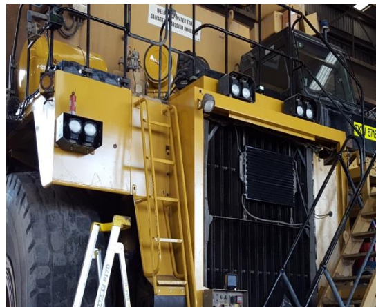
Replacement Mudguard and Radiator Cowling fabricated and fitted without any need for modification
