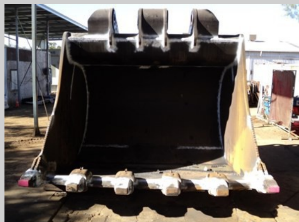
250 ton Excavator bucket rebuild including new adaptors & GET, heel plates, crack repairs & line boring.
