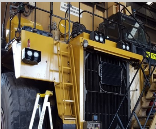
Replacement mudguard & radiator cowling fabricated & fitted.
