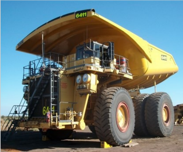
Komatsu 930E tray rebuild carried out on-site.
