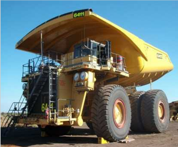
Komatsu 930E tray rebuild carried out on-site.
